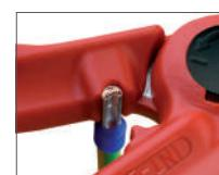
it crimps end-sleeves up to 4 mm<sup>2</sup>
